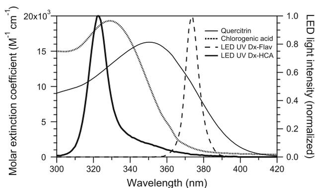
**Fig. 1** Spectra of molar extinction coefficients of chlorogenic acid in methanol and quercitrin (quercetin 3-*O*-rhamnoside) in 50/50 methanol/water (v/v) compared to the normalized spectra of the UV-light sources of the Dx-Flav and of the Dx-HCA
