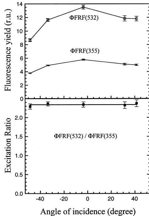
Fig. 7. Dependence of the FER on the angle of incidence. FRF, excited at 355 and 532 nm, and FER were measured on a tobacco leaf. The leaf was exposed at different angles of incidence, while the excitation beams and the detector remained at the same position. The error bars denote the standard deviation ( $N=170$ ).
