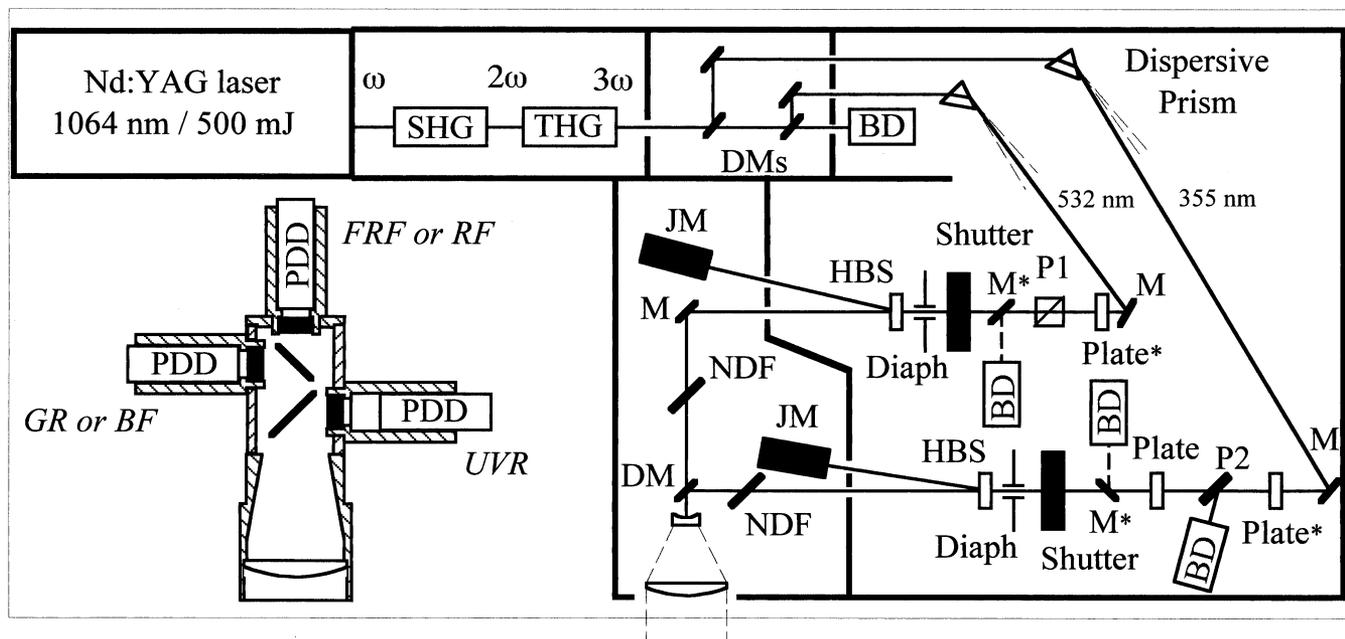
Fig. 1. Schematic diagram of the DE-FLIDAR. SHG: second harmonic generation; THG third harmonic generation; (\*) rotated by a step motor. For a detailed description, see Material, methods and instrumentation.
