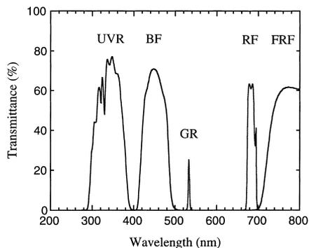
Fig. 2. Transmission spectra of the filter combinations used to protect the detectors and to define the spectral characteristics of fluorescence and reflectance signals. UVR: UV reflectance; GR: green reflectance; BF: blue fluorescence; FRF: far-red fluorescence; RF: red fluorescence.
