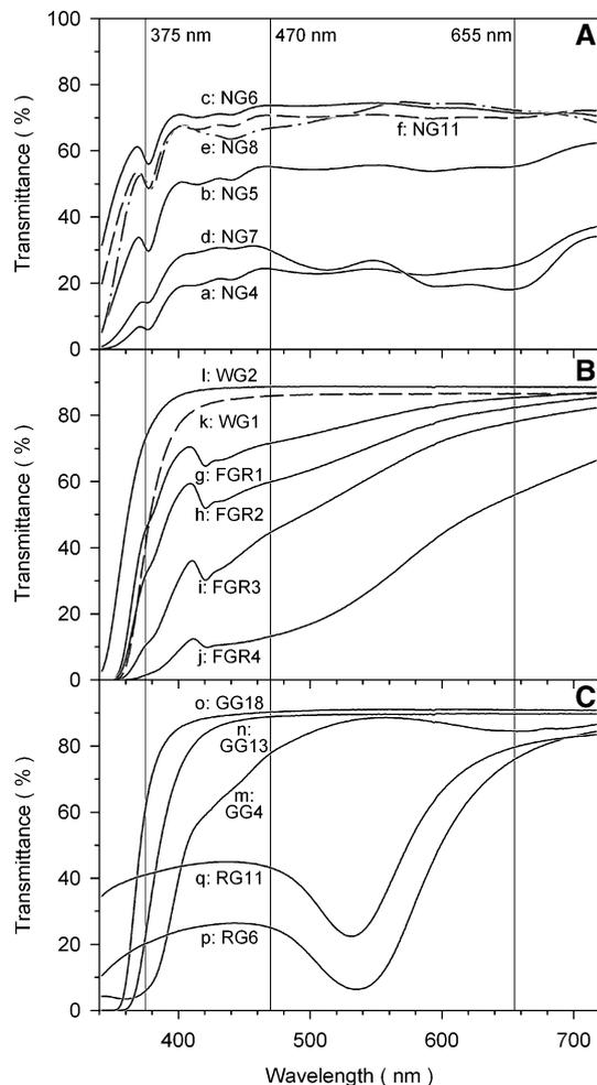
**Fig. 2** Transmittance spectra of glass filters. Transmittance spectra of glass filters that were employed to screen leaves. Spectra are labeled by the original filter designations together with small letters (a to q), which, in Figs. 3 and 4, indicate for each data point the filter used. Vertical lines specify the central wavelengths of fluorescence excitation (compare Fig. 1)
