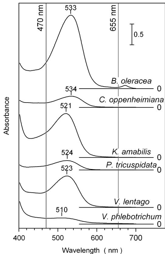
**Fig. 8** Absorbance spectra of acidic methanolic extracts of six red leaves. Original absorbance spectra and central wavelengths of visible excitation (vertical lines) by the Dualex and the UV-A-PAM fluorimeter are shown
