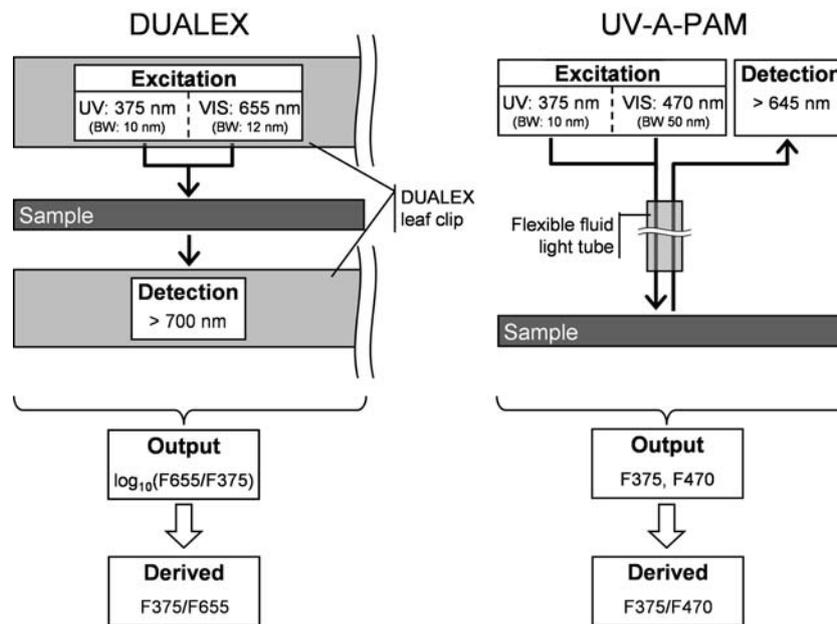
**Fig. 1** Key features of the Dualex and the UV-A-PAM fluorimeters. In the Dualex fluorimeter, samples are held by a leaf clip, and excitation and detection of fluorescence occur at opposite sides of the sample. The UV-A-PAM fluorimeter employs a flexible light guide as the optical connection between instrument and sample so that excitation and fluorescence detection occurs on the same side of the sample. Although
