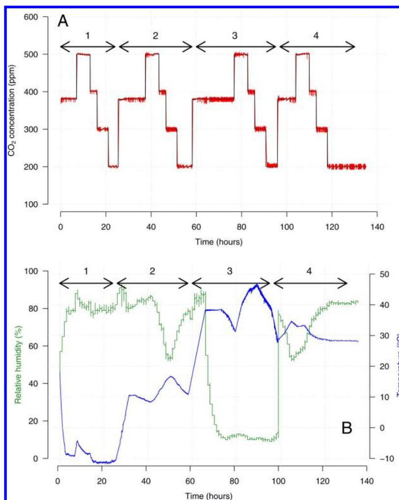
**Figure 3.** Efficiency of control of atmospheric CO<sub>2</sub> concentration (A), depending on climate conditions (B). (A) Measurements (red curve) and set-points (black curve) for set-points (black curve) at 380, 500, 400, 300, and 200 ppm. (B) Tests are repeated in four variable weather conditions: cold (1), temperate (2), hot and dry (3), and hot and humid weather (4).
