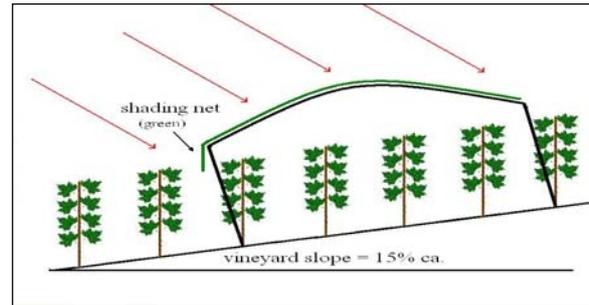
Figure 2: arrangement of the shading tunnel over the vineyard slope.
